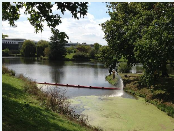
Barrage flottant – jupe antipollution Difope
